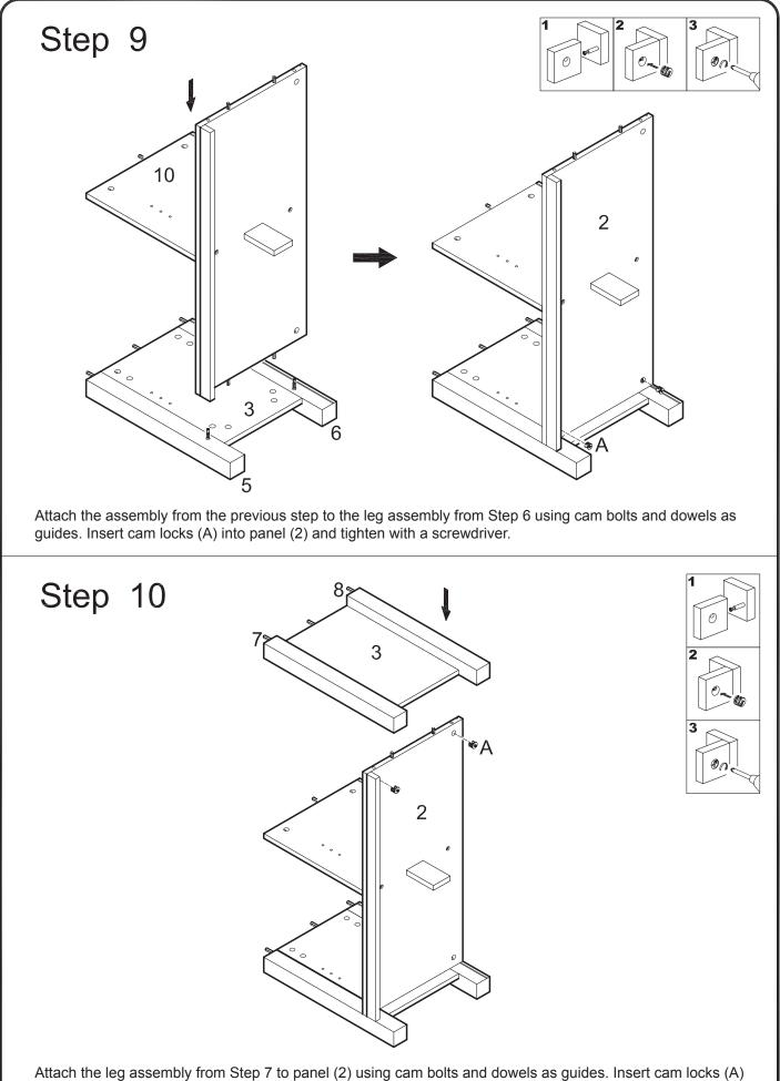
into panel (2) and tighten with a screwdriver.
